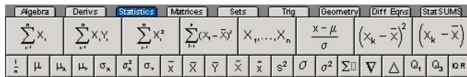
Figure 6: The Large Tabbed Bar (first row) and the Small Tabbed Bar (second row).
