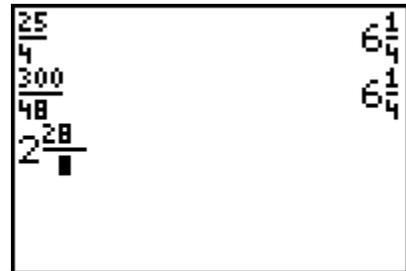
Figure 18: The whole number and the numerator for the simple fraction entered.
